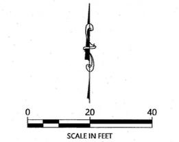
ORIENTATION OF THIS BEARING SYSTEM IS BASED ON THE MINNESOTA COUNTY COORDINATE SYSTEM, CASS COUNTY, NORTH ZONE (2011 ADJ.), ASSIGNING THE WEST LINE OF LOT 3 TO BEAR S00°34'21"W.
