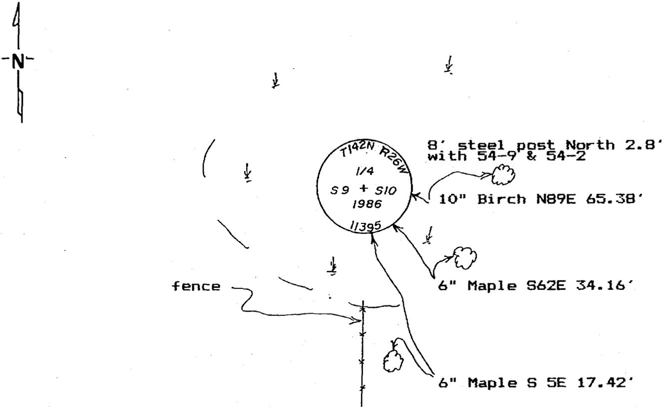
All measurements are to spks. in side of the tree, trees are double blazed and scribed and painted red with USFS 54-3 bearing tree tag.
