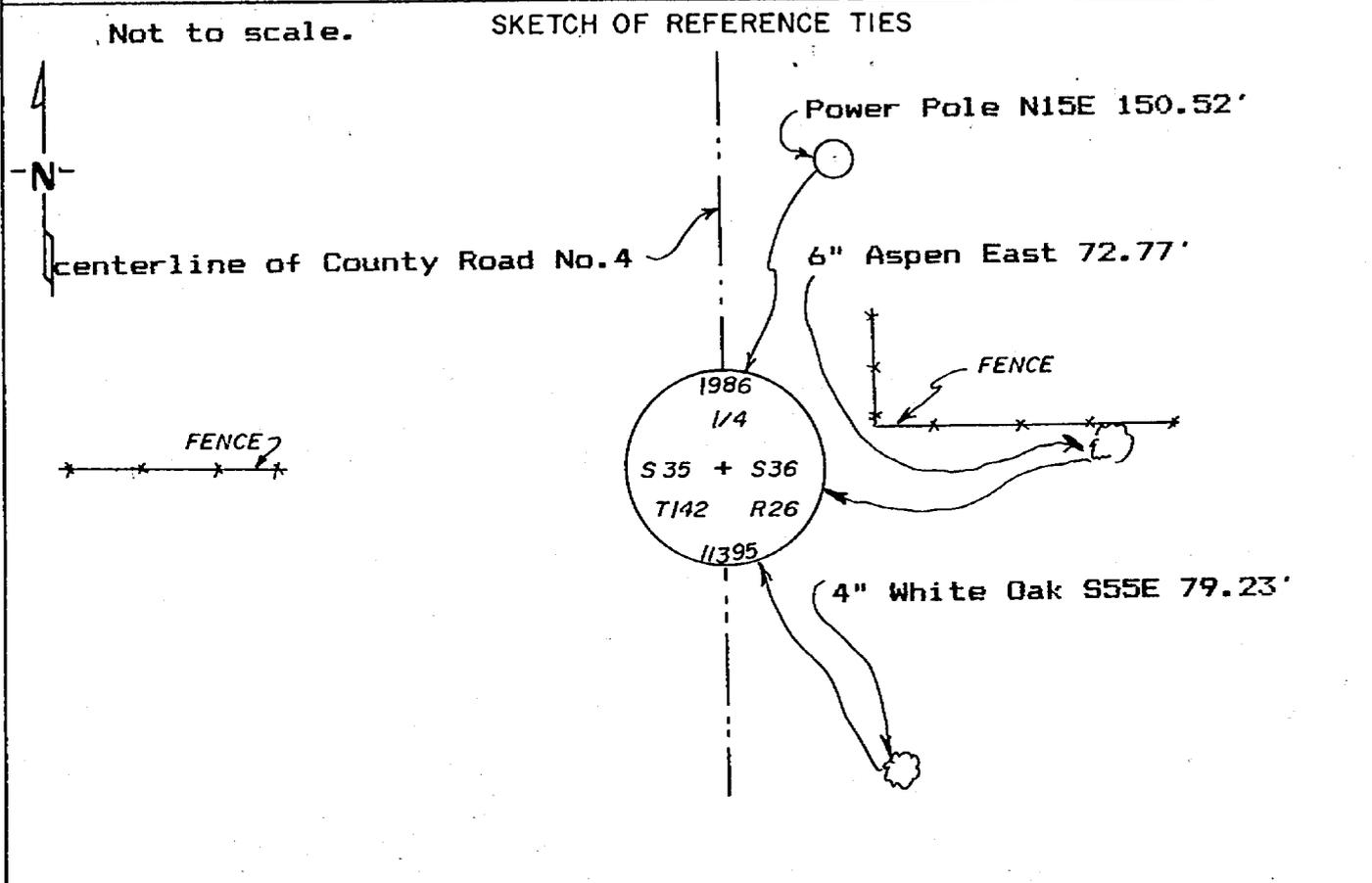
All measurements are to spks. in side of the tree, trees are double blazed and scribed and painted red with USFS 54-3 bearing tree tag.
