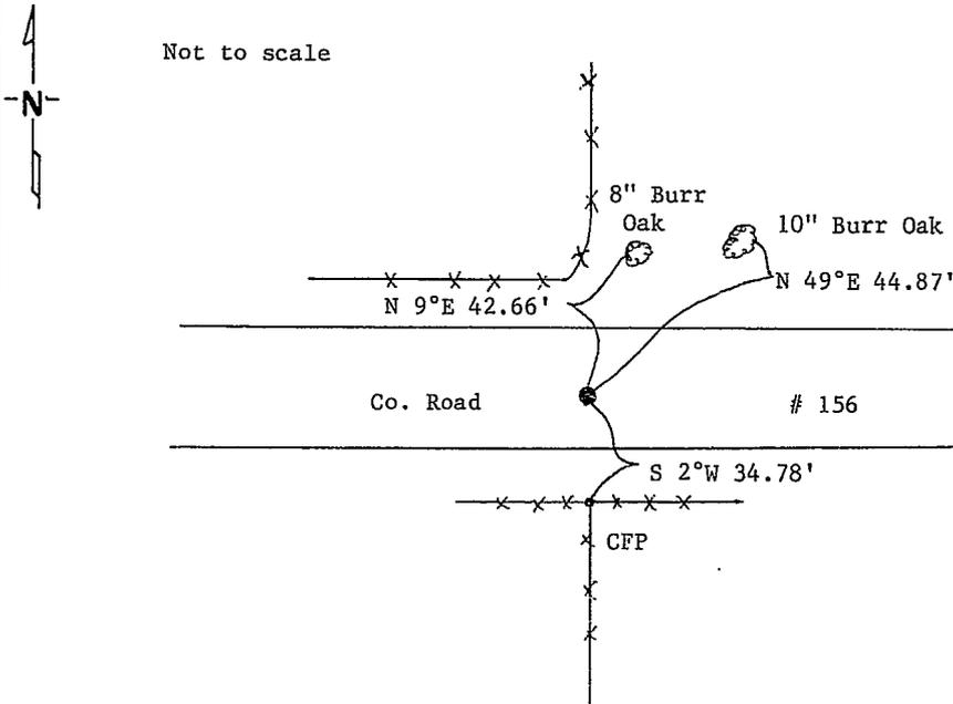
Measurements are to nail in side of object.
