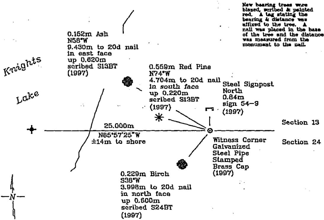
New bearing trees were blazed, scribed & painted red. A tag stating the bearing & distance was affixed to the tree. A nail was placed in the base of the tree and the distance was measured from the monument to the nail.
