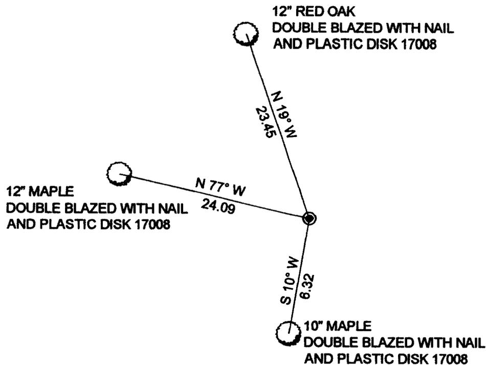
NOTE: DISTANCES SHOWN AS MEASURED TO NAIL IN SIDE OF FACE.
