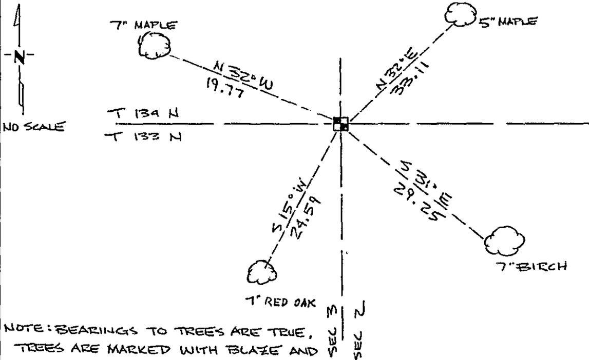
NOTE: BEARINGS TO TREES ARE TRUE, TREES ARE MARKED WITH BLAZE AND B.T. TAGS. DISTANCES ARE TO DUPLEX NAIL ON SIDE OF TREE. SIGN POST SET 1.0 NORTH OF MONUMENT.
