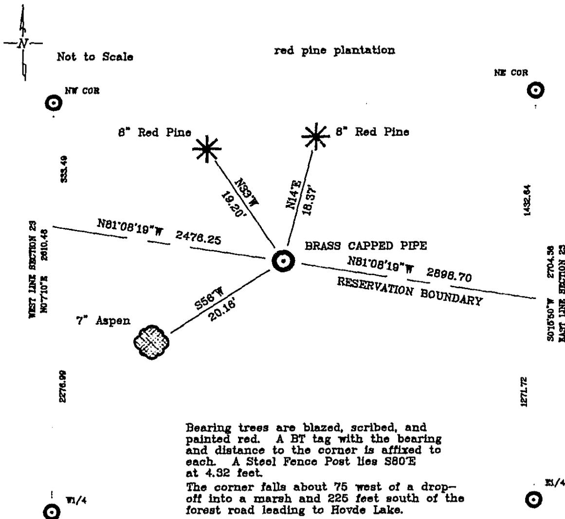
Bearing trees are blazed, scribed, and painted red. A BT tag with the bearing and distance to the corner is affixed to each. A Steel Fence Post lies S80°E at 4.32 feet.
