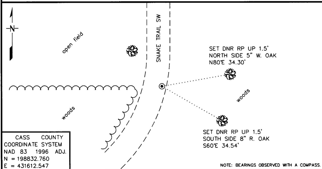
NOTE: BEARINGS OBSERVED WITH A COMPASS.
